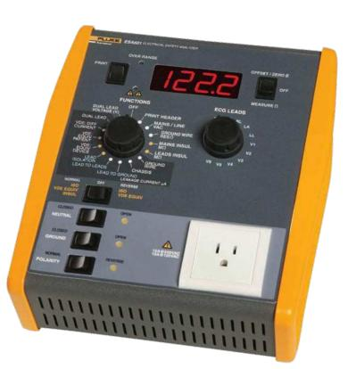
ESA601 Electrical Safety Analyzer tests medical equipment to both US and international standards. Users simply flip a switch to change between AAMI or IEC electrical safety testing load. The US version includes overlays in AAMI or IEC nomenclature so technicians use the terms that are most familiar to them. Multiple language overlays, outlets, and power cords are available for convenient use in many countries.
